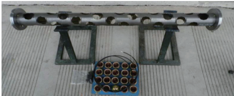
图 4 射孔弹与弹架管 Fig. 4 Perforating charges and carrier tube
